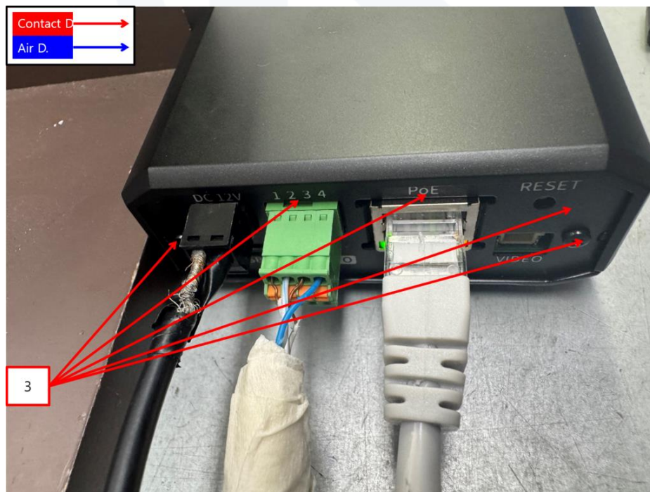
<Location of Discharge-2_Mode 1>
