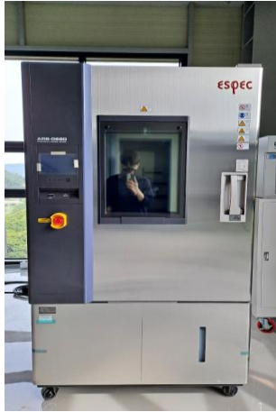
Temperature & Humidity Chamber
