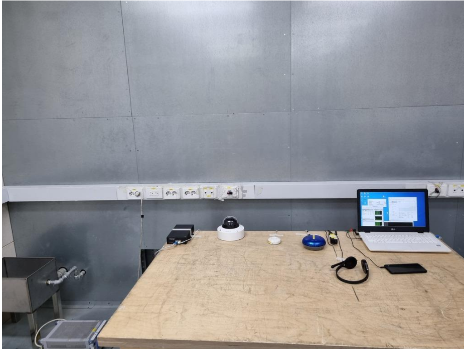
<Conducted Emissions at Telecommunication Ports - Front>
