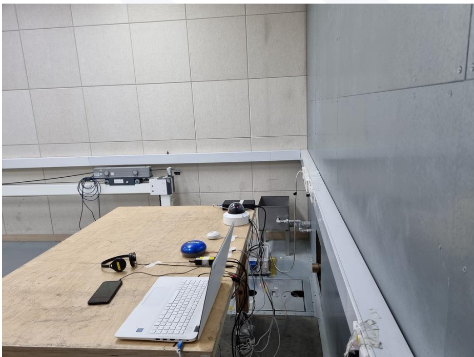
<Conducted Emissions at Telecommunication Ports - Rear>
