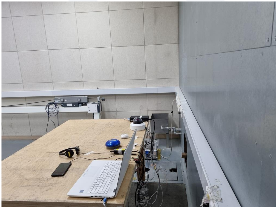
<Conducted Emissions at Telecommunication Ports - Rear>
