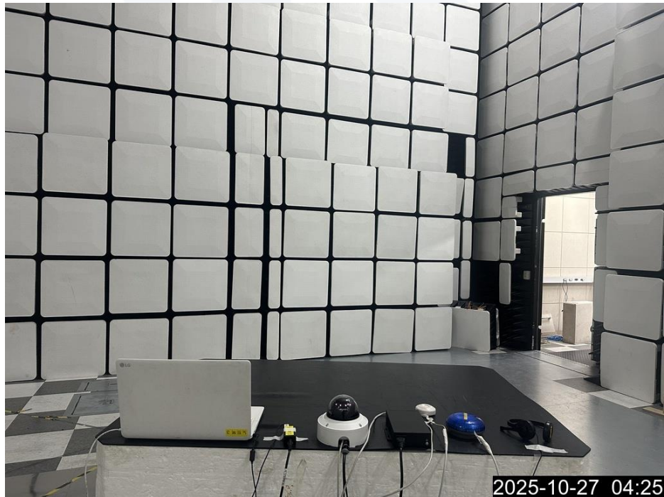
<Radiated Emissions(Below 1 GHz) - Rear> Mode 2
