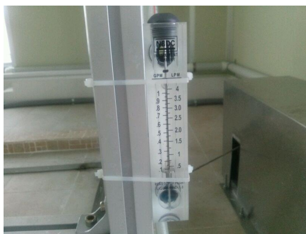
Water flow meter with Drip box
