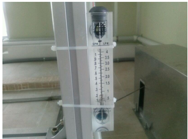
Water flow meter with Drip box
