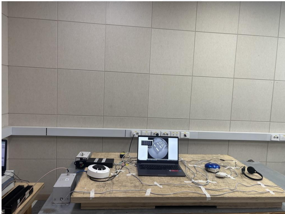
<Continuous Induced RF Disturbances> Mode 2
