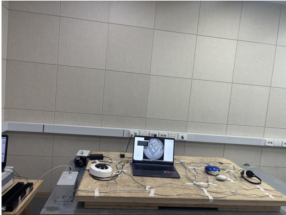
<Continuous Induced RF Disturbances> Mode 1
