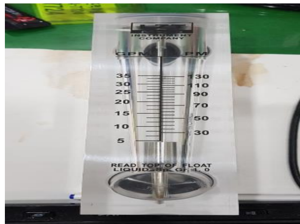
Water flow meter with IPX6
