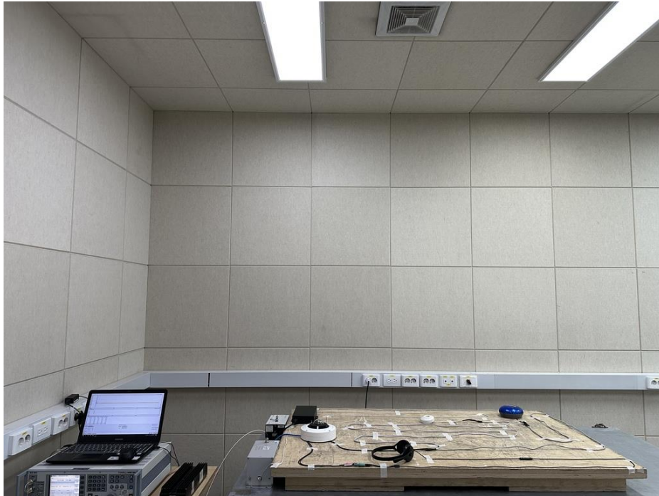
<Continuous Induced RF Disturbances> Mode 2
