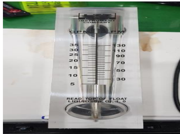
Water flow meter with IPX6
