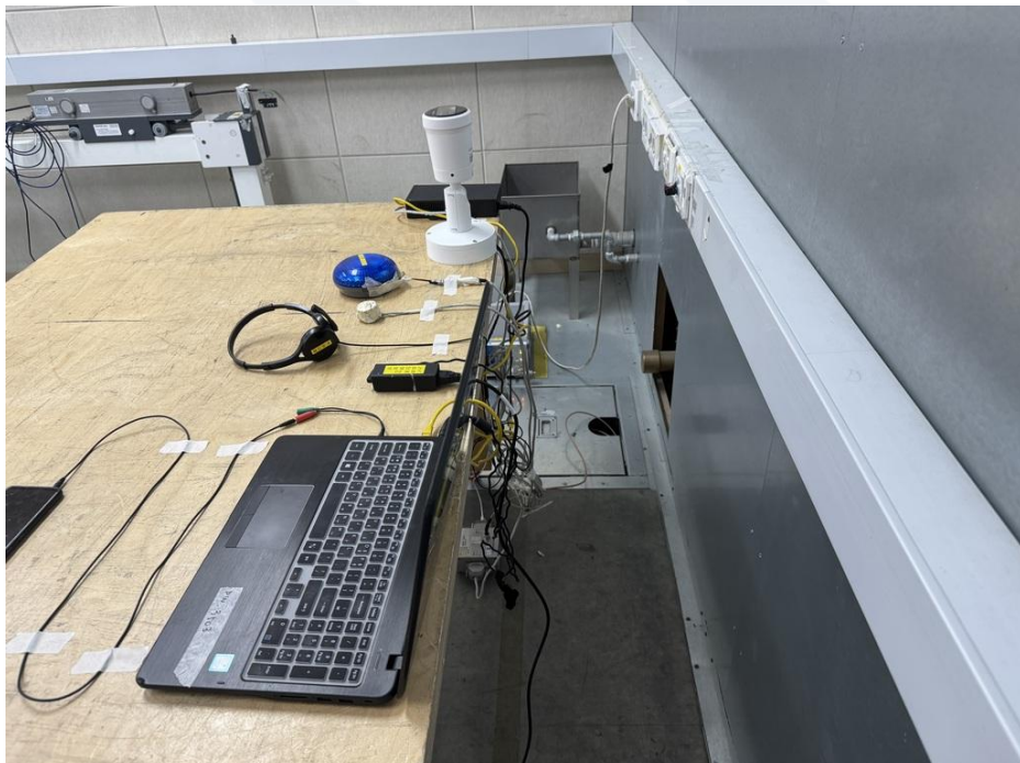
<Conducted Emissions at Telecommunication Ports - Rear>
