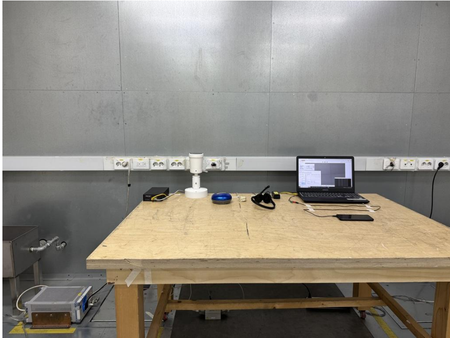
<Conducted Emissions at Telecommunication Ports - Front>
