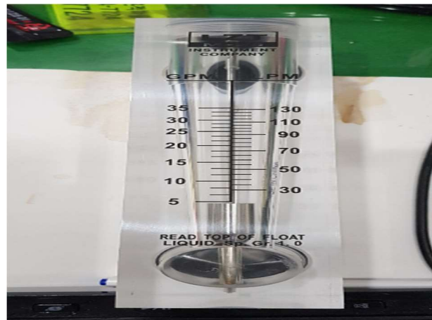
Water flow meter with IPX6
