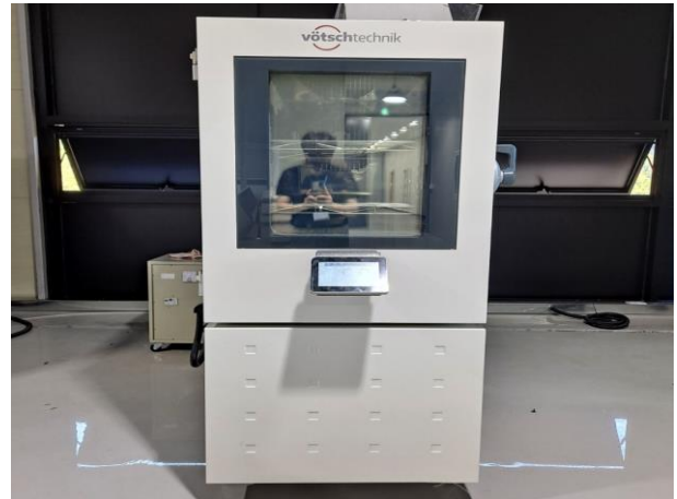
Temperature & Humidity Chamber
