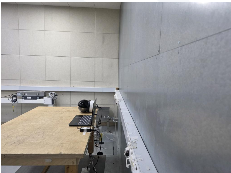
<Conducted Emissions at Telecommunication Ports - Rear>
