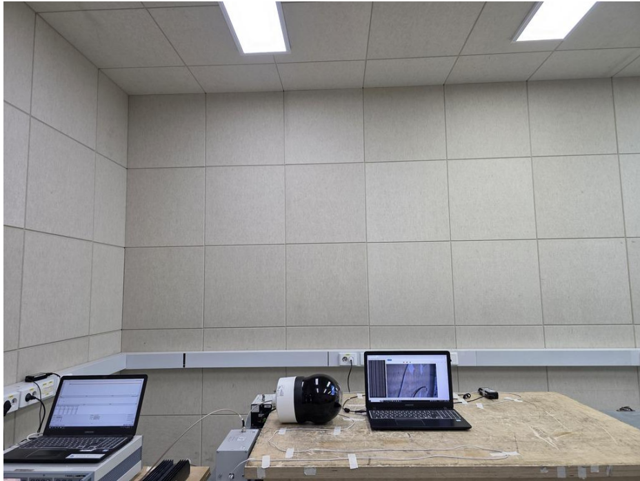
<Continuous Induced RF Disturbances>
