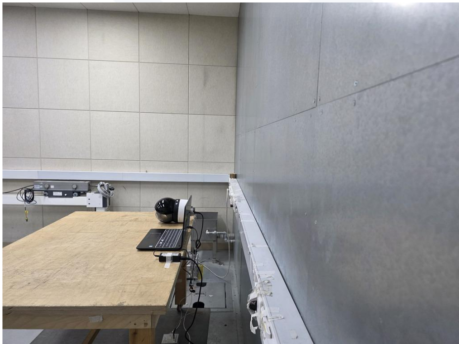
<Conducted Emissions at Telecommunication Ports - Rear>
