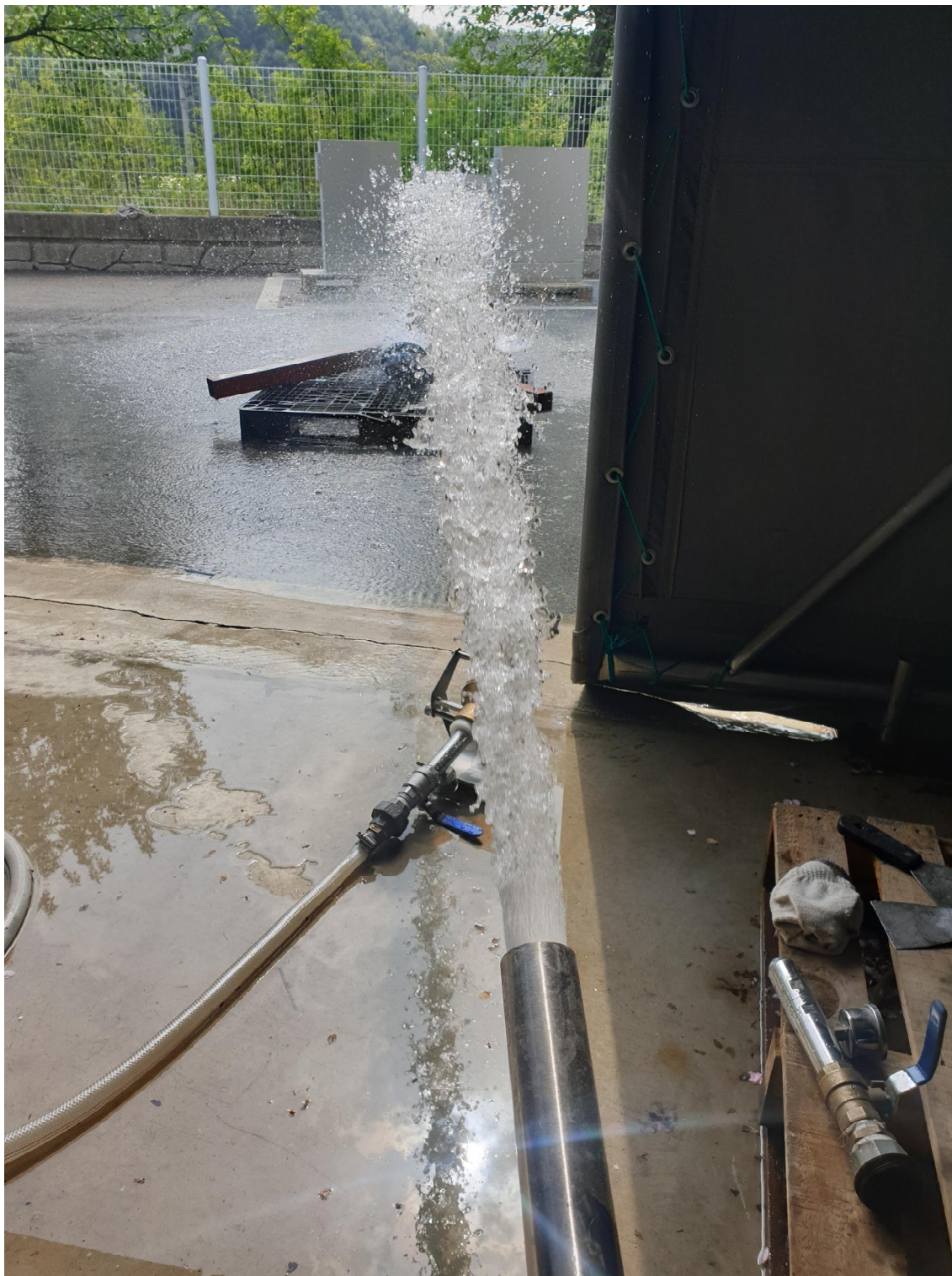
<Photo 3 > Hose down test
