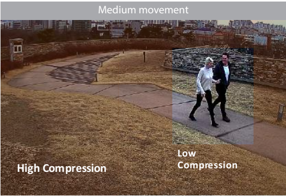
WiseStream II OFF : 7260kbps WiseStream II ON : 1817kbps
