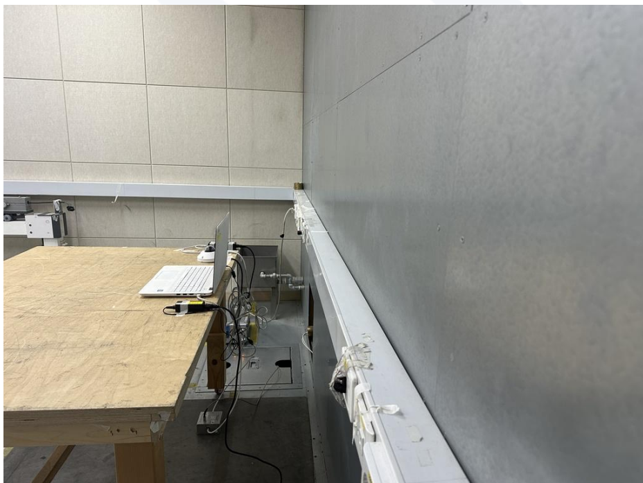
<Conducted Emissions at Telecommunication Ports - Rear>
