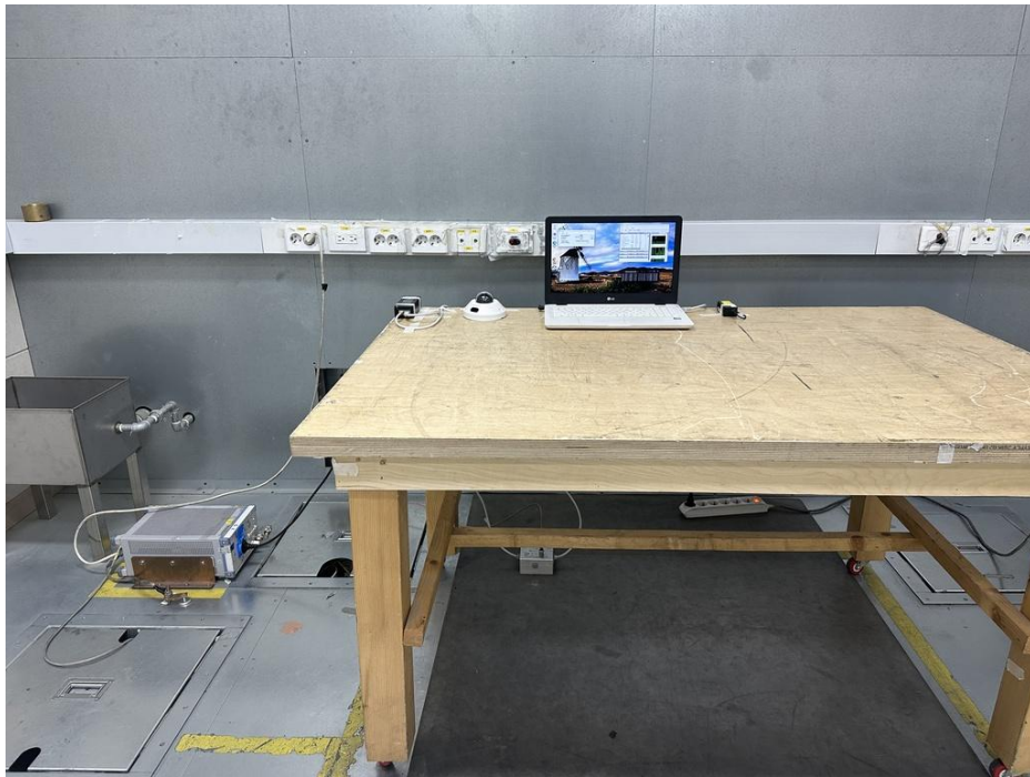
<Conducted Emissions at Telecommunication Ports - Front>
