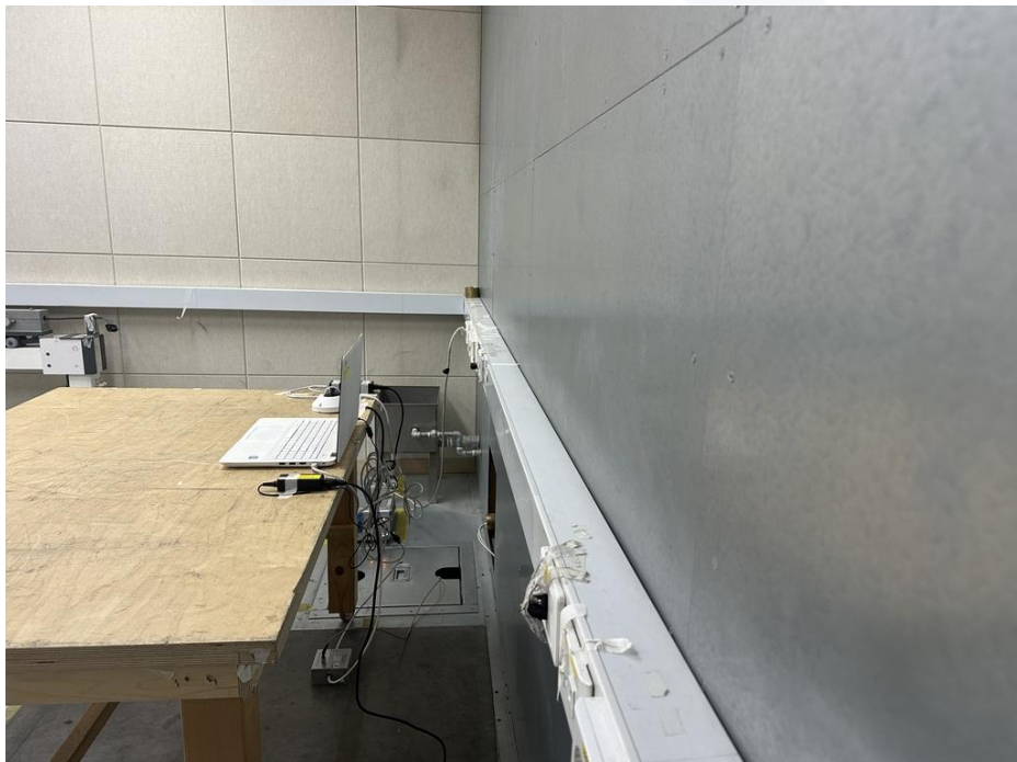
<Conducted Emissions at Telecommunication Ports - Rear>
