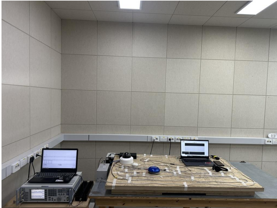
<Continuous Induced RF Disturbances>
