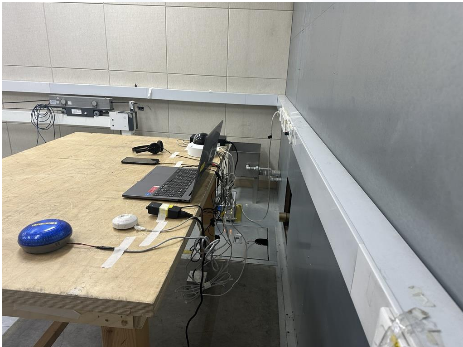
<Conducted Emissions at Telecommunication Ports - Rear>
