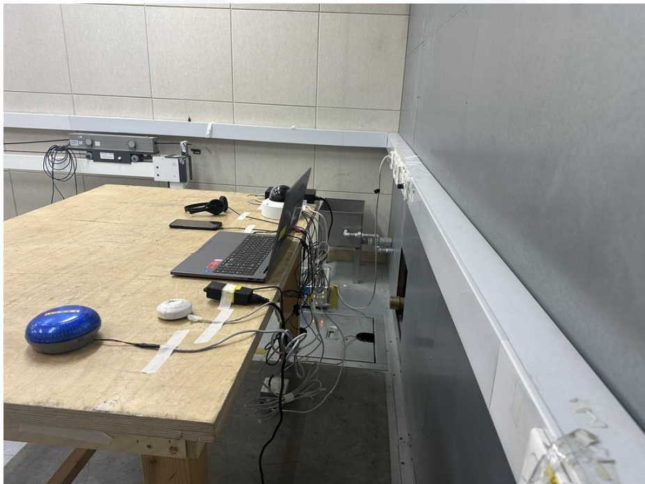
<Conducted Emissions at Telecommunication Ports - Rear>
