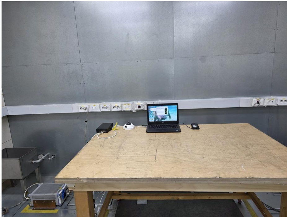
<Conducted Emissions at Telecommunication Ports - Front>
