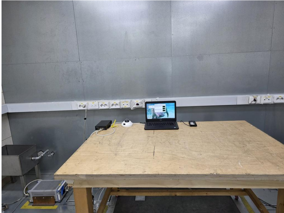
<Conducted Emissions at Telecommunication Ports - Front>
