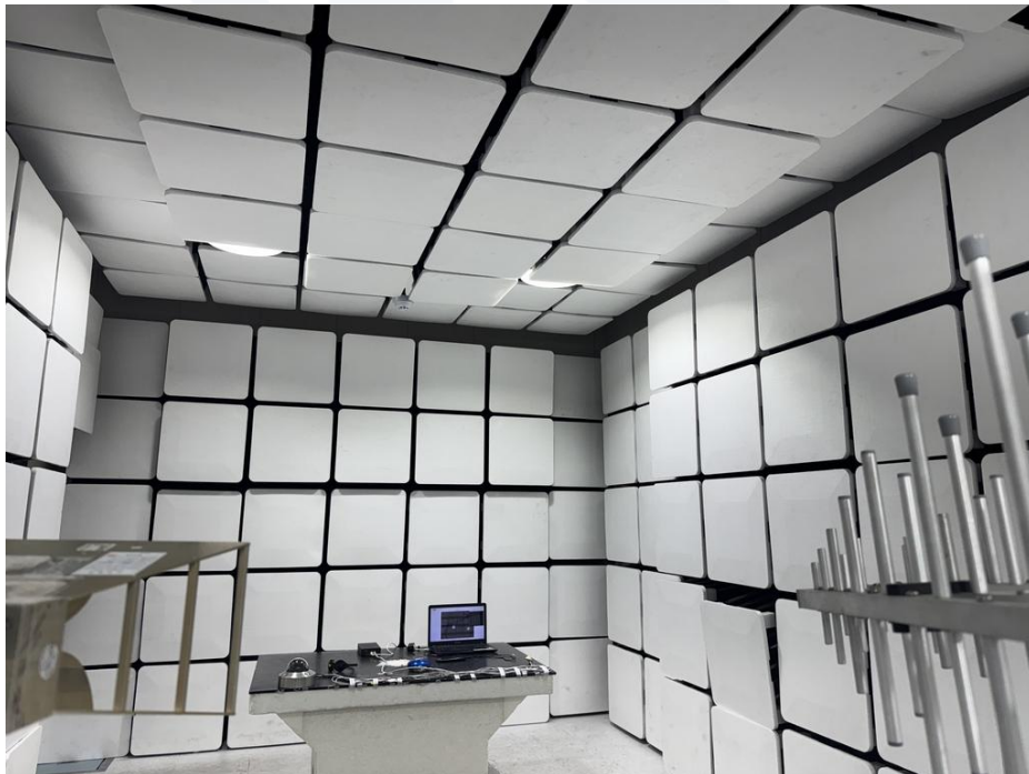
<Continuous RF electromagnetic field disturbances>
