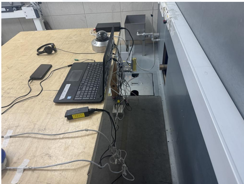
<Conducted Emissions at Telecommunication Ports - Rear>
