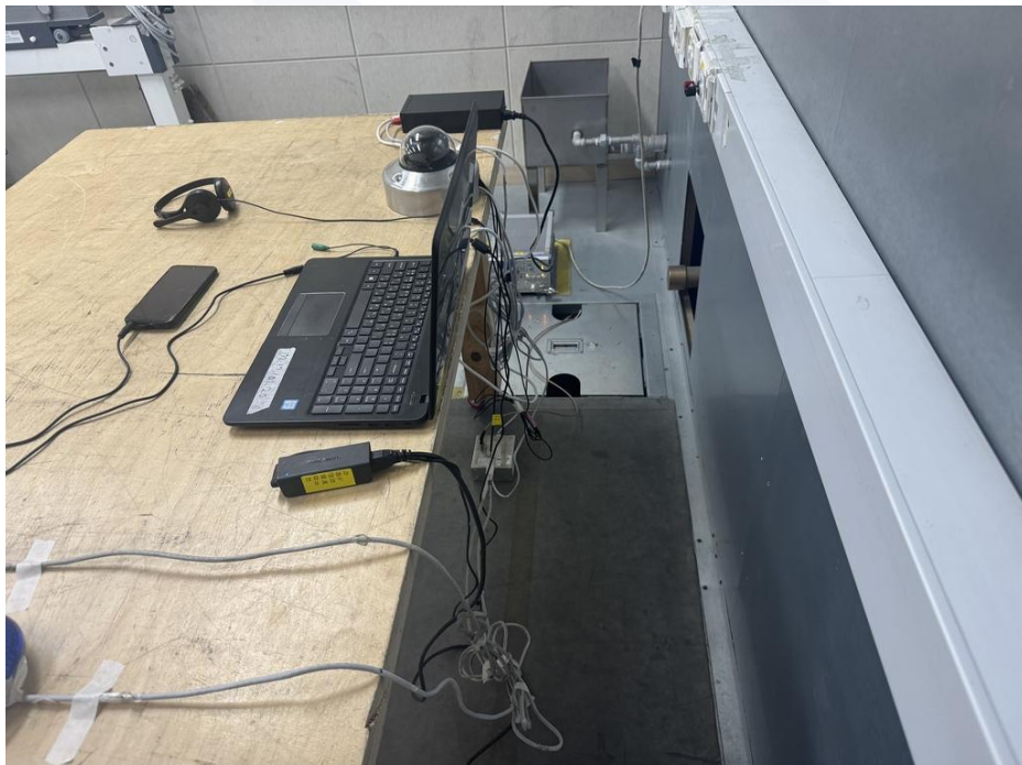
<Conducted Emissions at Telecommunication Ports - Rear>
