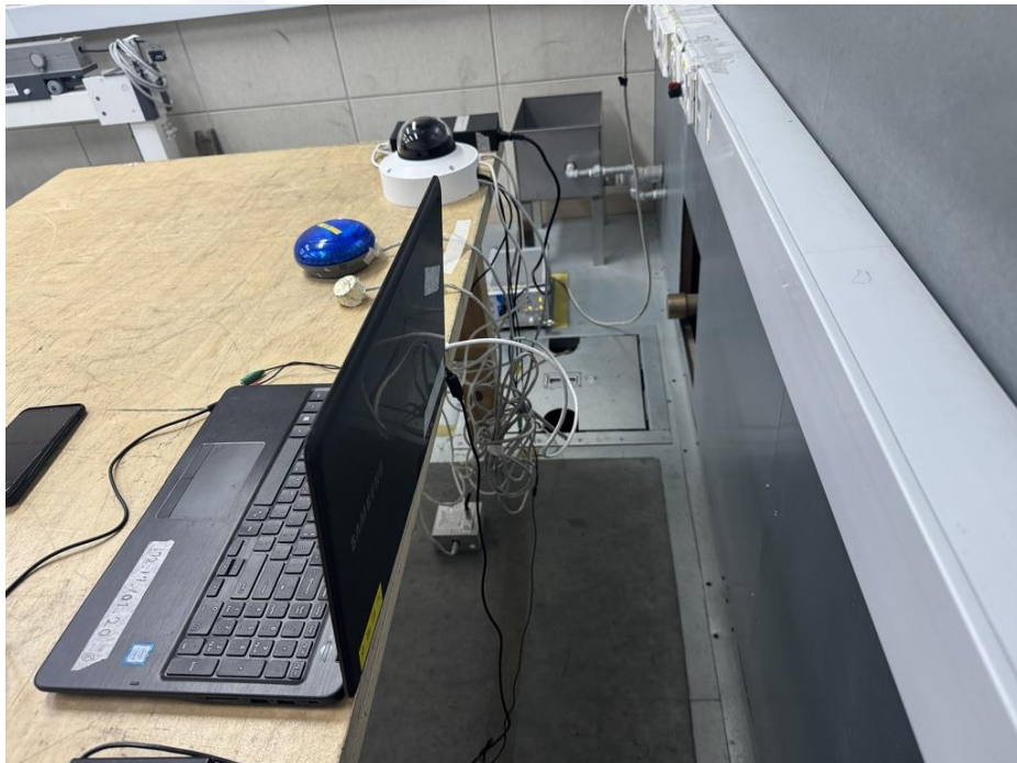
<Conducted Emissions at Telecommunication Ports - Rear> Mode 2
