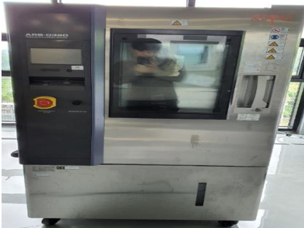
Temperature & Humidity Chamber
