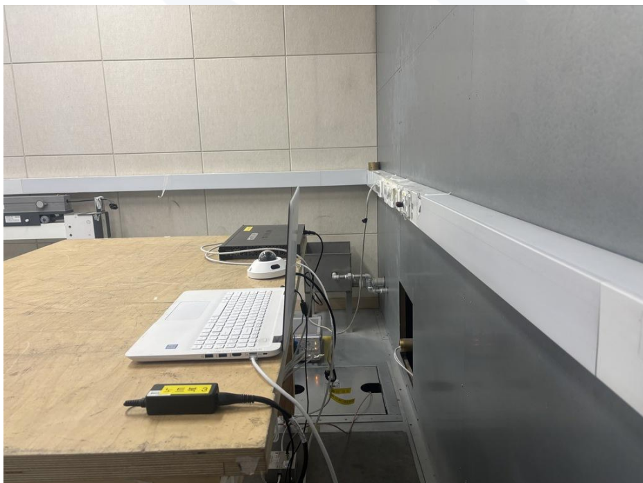
<Conducted Emissions at Telecommunication Ports - Rear>
