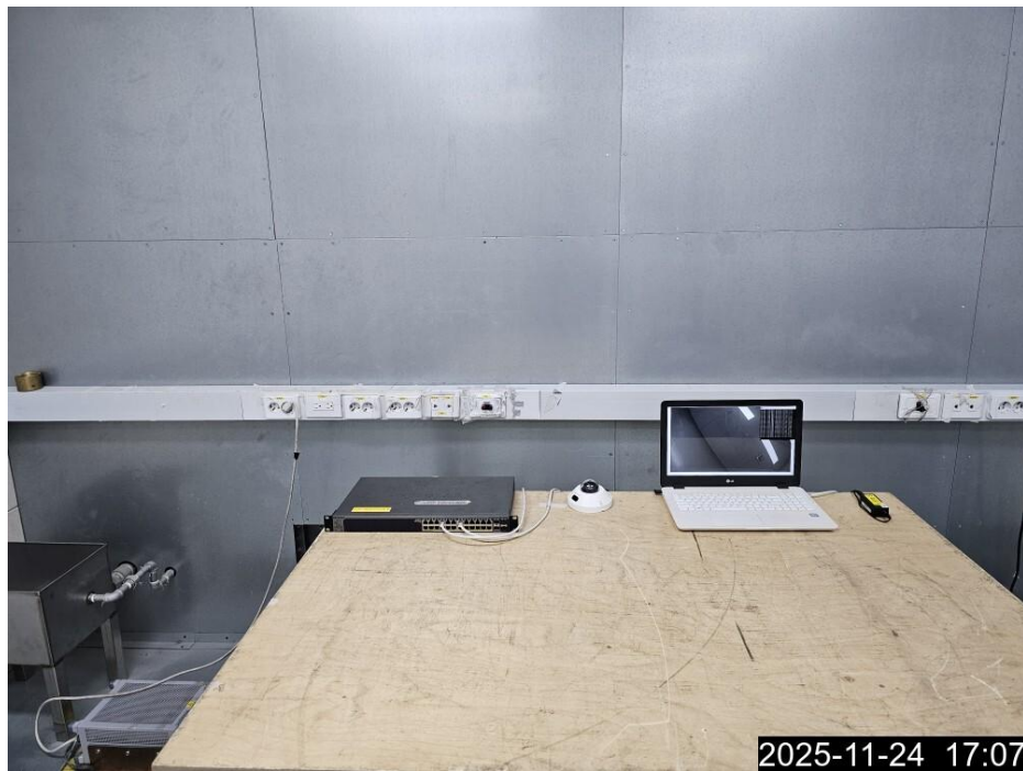
<Conducted Emissions at Mains Power Ports - Front>
