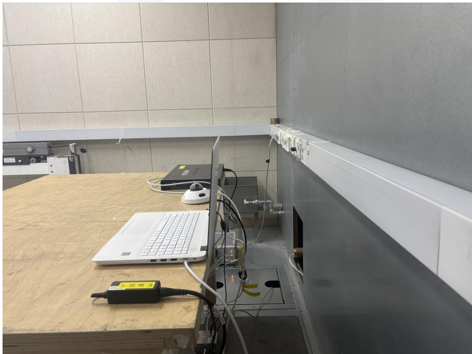
<Conducted Emissions at Telecommunication Ports - Rear>
