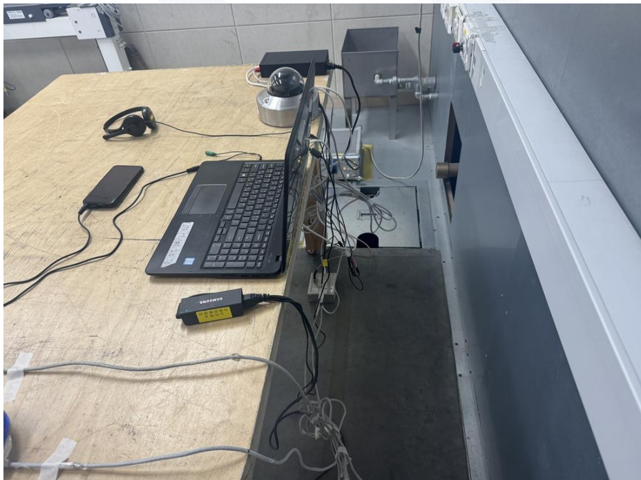
<Conducted Emissions at Telecommunication Ports - Rear>
