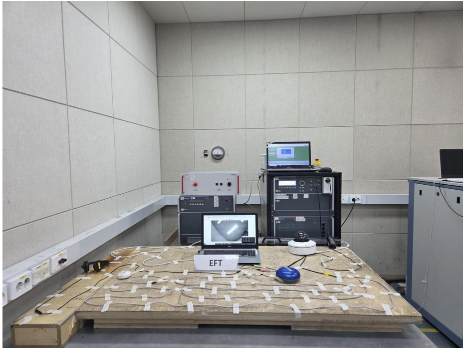
<Electrical Fast Transients/Bursts> Mode 1
