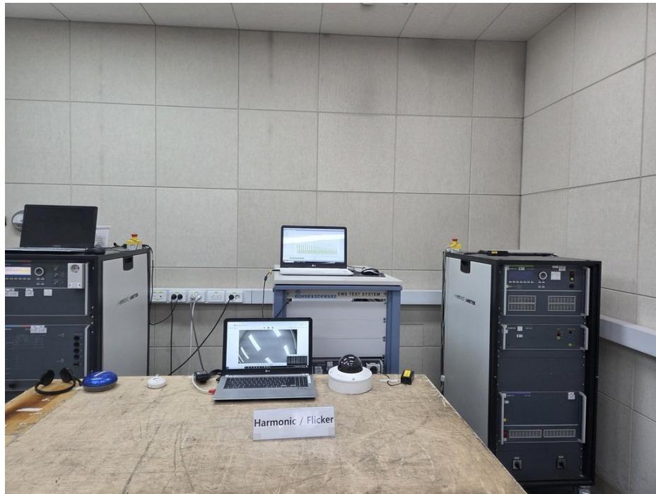
<Harmonic Current Emissions and Voltage Fluctuations and Flicker> Mode 1
