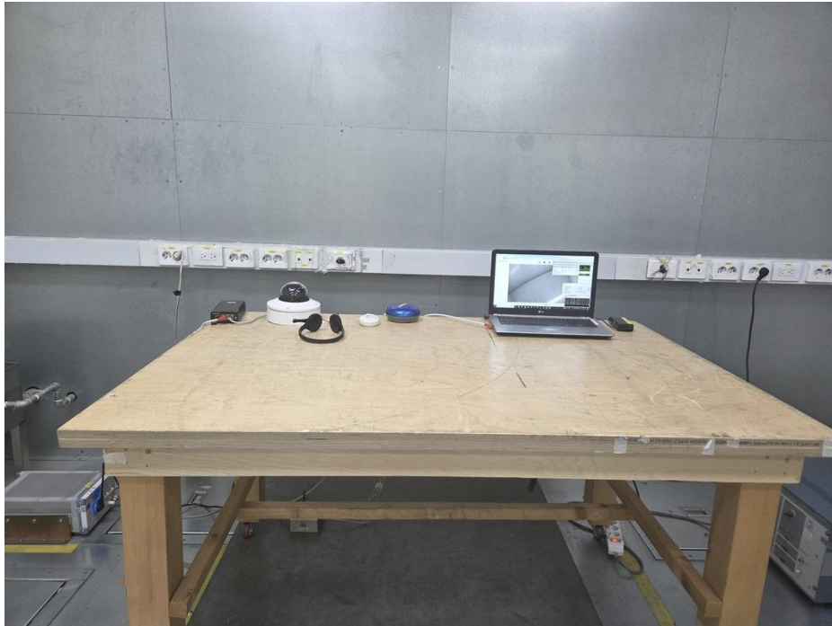
<Conducted Emissions at Telecommunication Ports - Front>Mode 2
