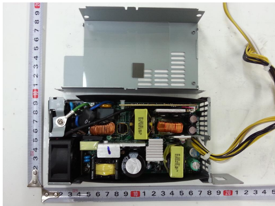
<Photo 14 > Inside – SMPS
